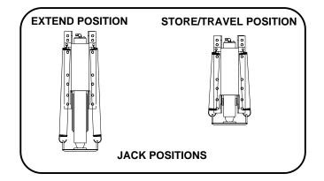
**CAUTION:** DO NOT MOVE THE VEHICLE WHILE THE LEVELING JACKS ARE STILL IN CONTACT WITH THE GROUND OR IN THE EXTEND POSITION. THIS VEHICLE IS EQUIPPED WITH STRAIGHT-ACTING JACKS. MOVING THE VEHICLE WITH THE LEVELING JACKS EXTENDED CAN CAUSE SEVER DAMAGE TO THE JACKS AND OR THE VEHICLE AND CREATE A DRIVING HAZARD. DO NOT RELY SOLELY UPON WARNING LIGHTS. IT IS THE OPERATOR'S RESPONSIBILITY TO CHECK THAT ALL JACKS ARE FULLY RETRACTED INTO THE STORE/ TRAVEL POSITION.
