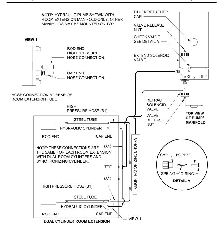
**IMPORTANT:** THE LINES (A1) BETWEEN THE CAP END OF THE HYDRAULIC CYLINDERS AND THE TEE MUST BE THE SAME LENGTH AND DIAMETER.
