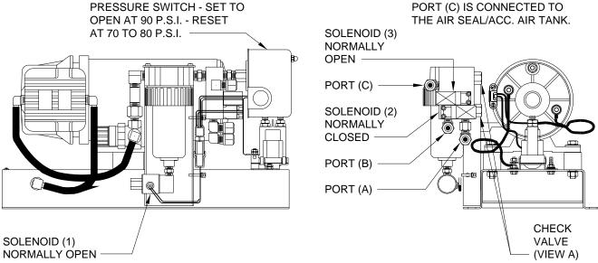
SOLENOID (1) IS THE WATER TRAP DUMP VALVE. THIS VALVE IS CLOSED WHENEVER THE COMPRESSOR IS RUNNING.
