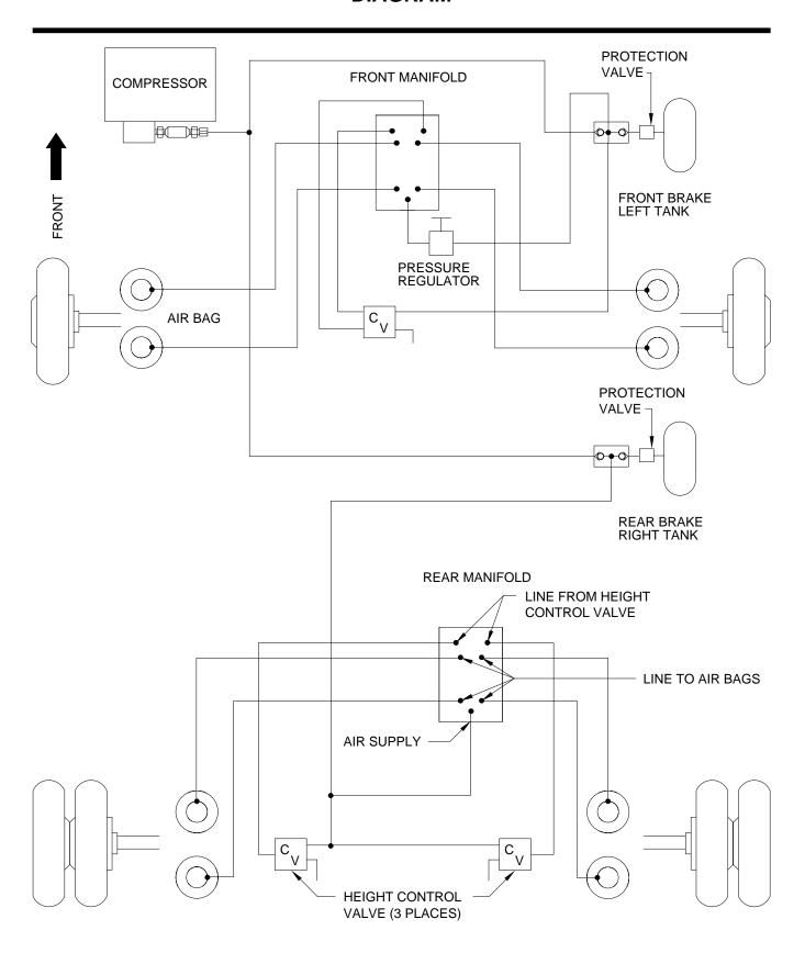
MANIFOLDS ARE MOUNTED TO MAIN CROSS MEMBERS. LEAVE AMPLE CLEARANCE FOR CONNECTION OF HOSES TO FITTINGS.
